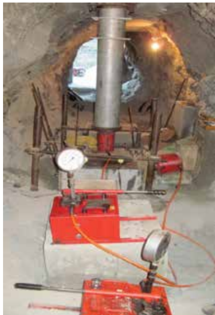
Figure 2 Photograph of shear test set-up Figure 3 Schematic diagram of shear test set up
