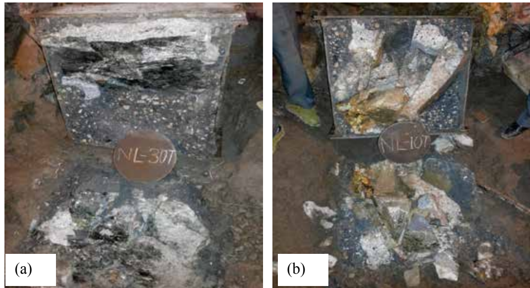
Figure 6 Overturned rock blocks tested at normal load (a) 30T and (b) 10T
